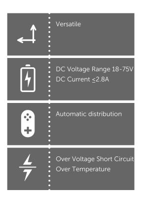
Current Splitter is designed to save costs on Led Drivers and mainly on installation. The unit divides the total Amperage from the driver into 2,3,4 channels/strings depending on the fixture. Maximum efficiency for the system can be achieved by using the current splitter for 4 channels/Strings
